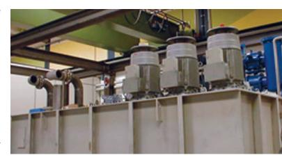
system manufacturer and choosing the NSSV, Colfax has ensured that only the pumps get replaced; the original motors are remounted to the replacement pumps, further minimizing the effort and costs associated with the retrofit.
